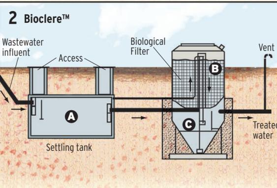
Bioclere combines a filter with a water clarifier in a unique configuration, said Craig Lindell, chief executive officer of AquaPoint, the company that produces the system. Like many systems, it separates most of the solids in the wastewater stream in a settling tank (A) and then uses a biological filter (B) in which micro organisms feed on the nitrogen. But unlike other systems the filter is located on top of a (C) clarifier. Bioclere is also available only on a provisional-use basis.
