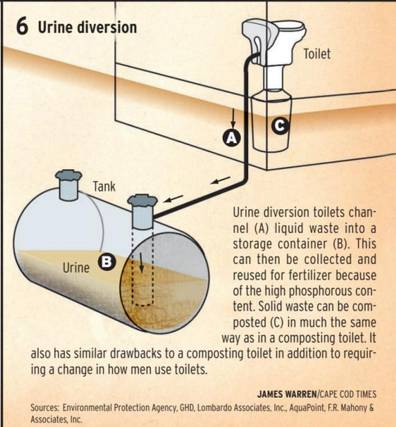
Urine diversion toilets channel (A) liquid waste into a storage container (B). This can then be collected and reused for fertilizer because of the high phosphorous content. Solid waste can be composted (C) in much the same way as in a composting toilet. It also has similar drawbacks to a composting toilet in addition to requiring a change in how men use toilets.
