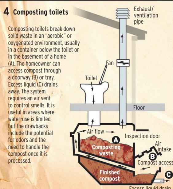
Composting toilets break down solid waste in an "aerobic" or oxygenated environment, usually in a container below the toilet or in the basement of a home (A). The homeowner can access compost through a doorway (B) or tray. Excess liquid (C) drains away. The system requires an air vent to control smells. It is useful in areas where water-use is limited but the drawbacks include the potential for odors and the need to handle the compost once it is processed.
