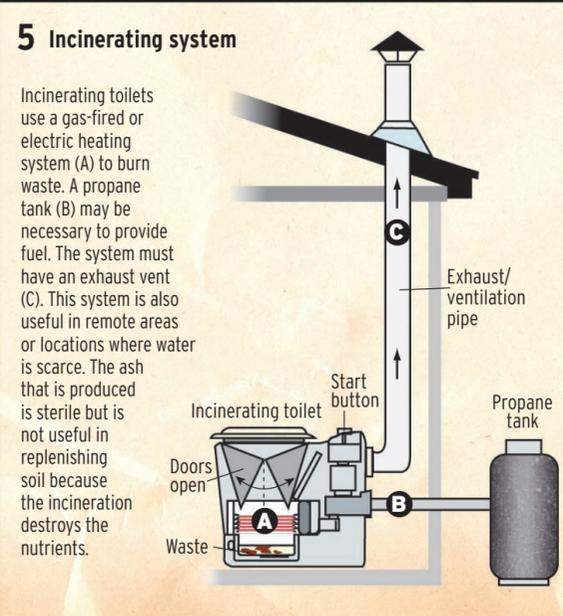
Incinerating toilets use a gas-fired or electric heating system (A) to burn waste. A propane tank (B) may be necessary to provide fuel. The system must have an exhaust vent (C). This system is also useful in remote areas or locations where water is scarce. The ash that is produced is sterile but is not useful in replenishing soil because the incineration destroys the nutrients.
